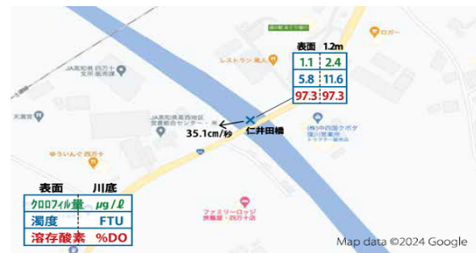
Chlorophyll amount turbidity and dissolved oxygen and flow direction, velocity under Niida Bridge, 12 May 2024
