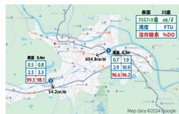
Chlorophyll amount, turbidity, dissolved oxygen, flow direction and velocity of the Nara River, 13 May 2024
