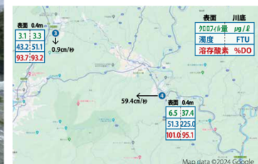
Chlorophyll amount, turbidity, dissolved oxygen, flow direction and velocity of the Mima River, 13 May 2024
